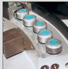
Adjustable bearing design
